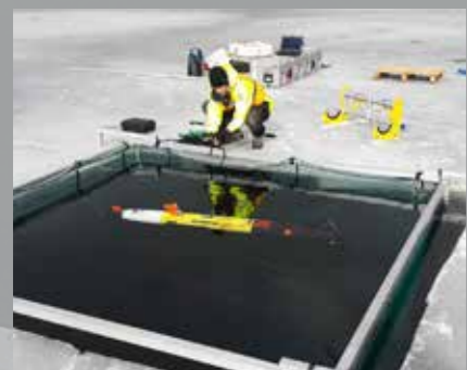
A PhD fellow prepares an autonomous subsea vessel (AUV) for operation under ice.
