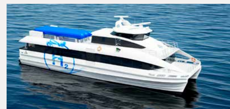
Artist's rendering of how the world's first hydrogen powered high-speed craft might look if HRF members Brødrene Aa, Florø Skyssebåt and MANCRAFT succeed. Note the hydrogen tanks and associated equipment placed on the upper deck.
