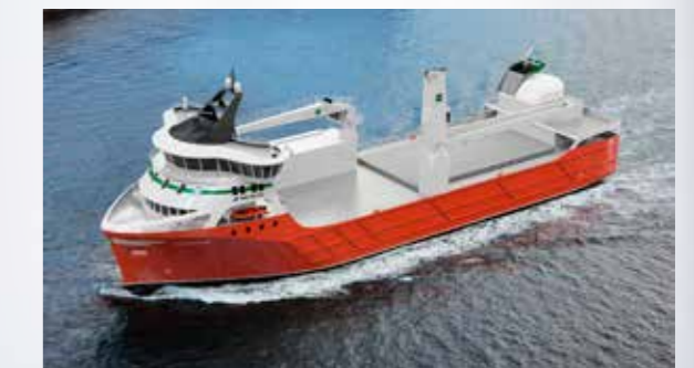
THE NEW KRISTIAN WITH – a hybrid LNG and battery vessel – is one of the pilot projects in phase 2 of the Green Coastal Shipping Programme. This project is owned by Kystrederiene.
