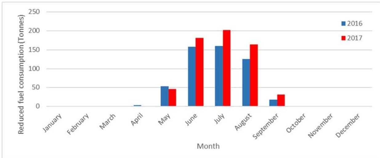
**Figure 3-4 Distribution of monthly fuel consumption reduction potentials, with a speed limit of 8 knots, based on 2016 and 2017 data. Source DNV GL**
