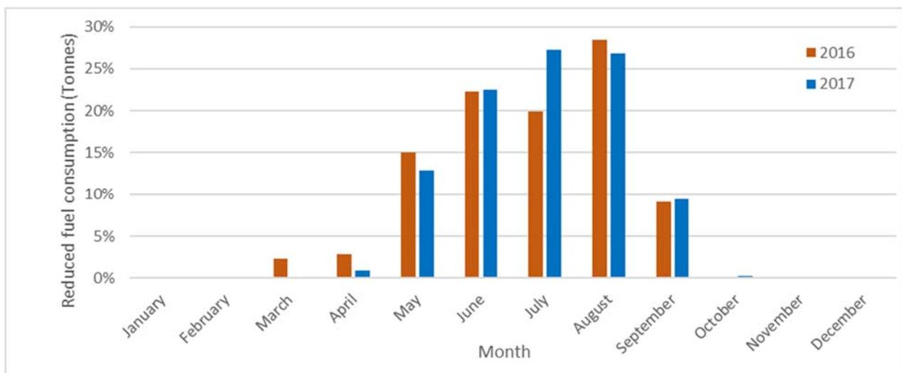
**Figure 3-7 Distribution of monthly fuel consumption reduction potentials, with a speed limit of 8 knots, based on 2016 and 2017 data. Source DNV GL**
