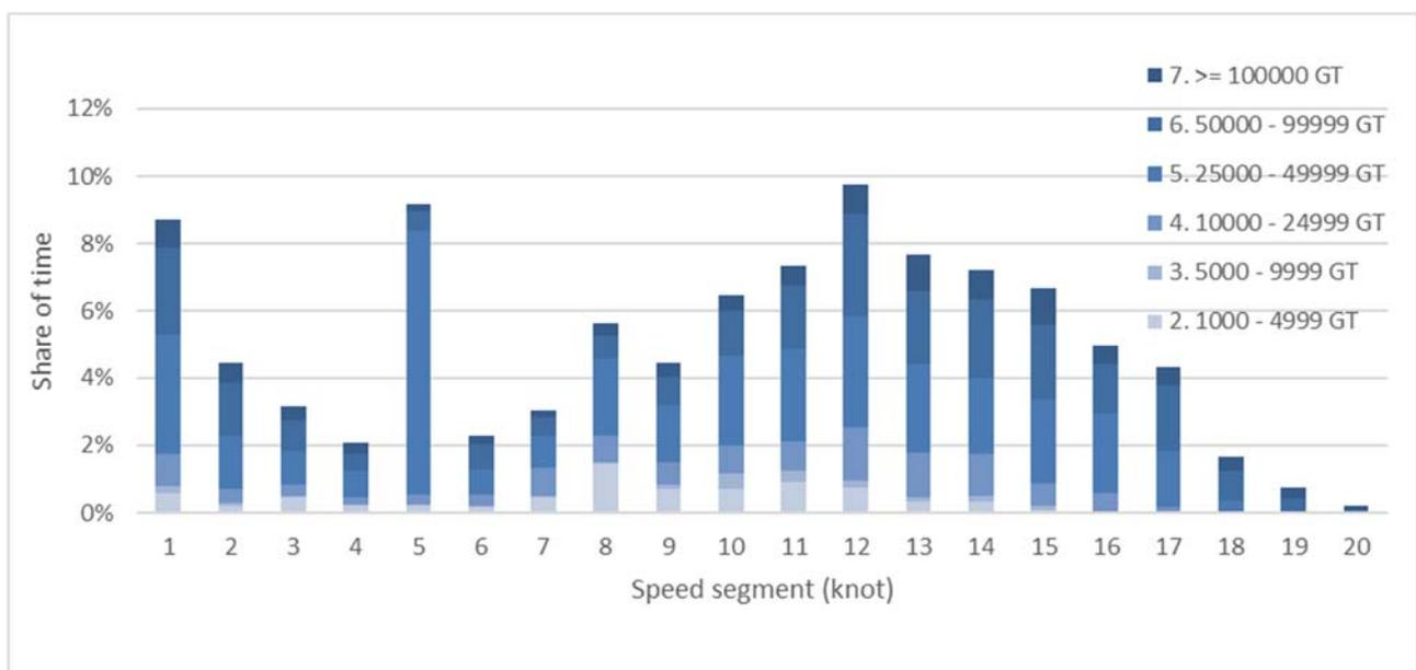
**Figure 3-5 Speed profile for different vessel size categories operating in Aurlandsfjord and Nærøyfjord. Source DNV GL**
