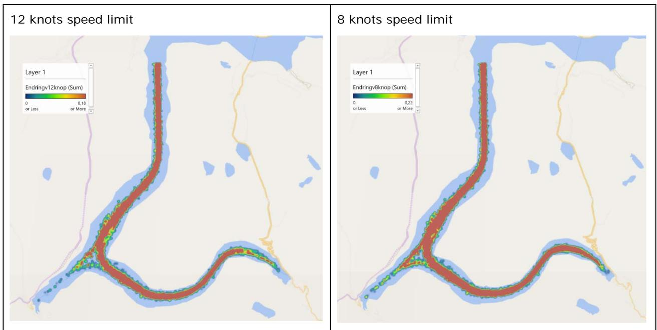
**Figure 3-3 Emission reduction areas based on speed limits of 12 knots (left) and 8 knots (right). Source DNV GL**
