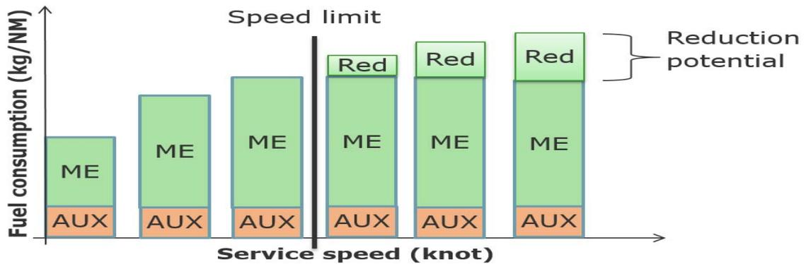
**Figure 2-1 Principle for estimating emission reduction potentials introducing speed limits**
