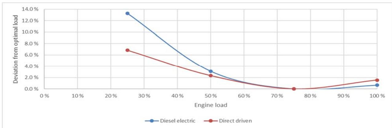
**Figure 2-2 Deviation in specific fuel oil consumption from optimal load. Source: DNV GL**
