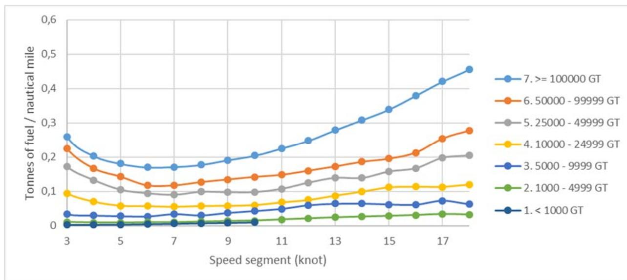
Figure 3-2 Fuel consumption for different speeds and size categories of ship. Source DNV GL
