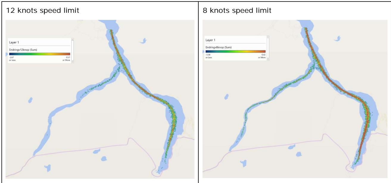
**Figure 3-6 Area of influence for potential emission reduction with speed limits of 12 knots (left) and 8 knots (right). Source DNV GL**
